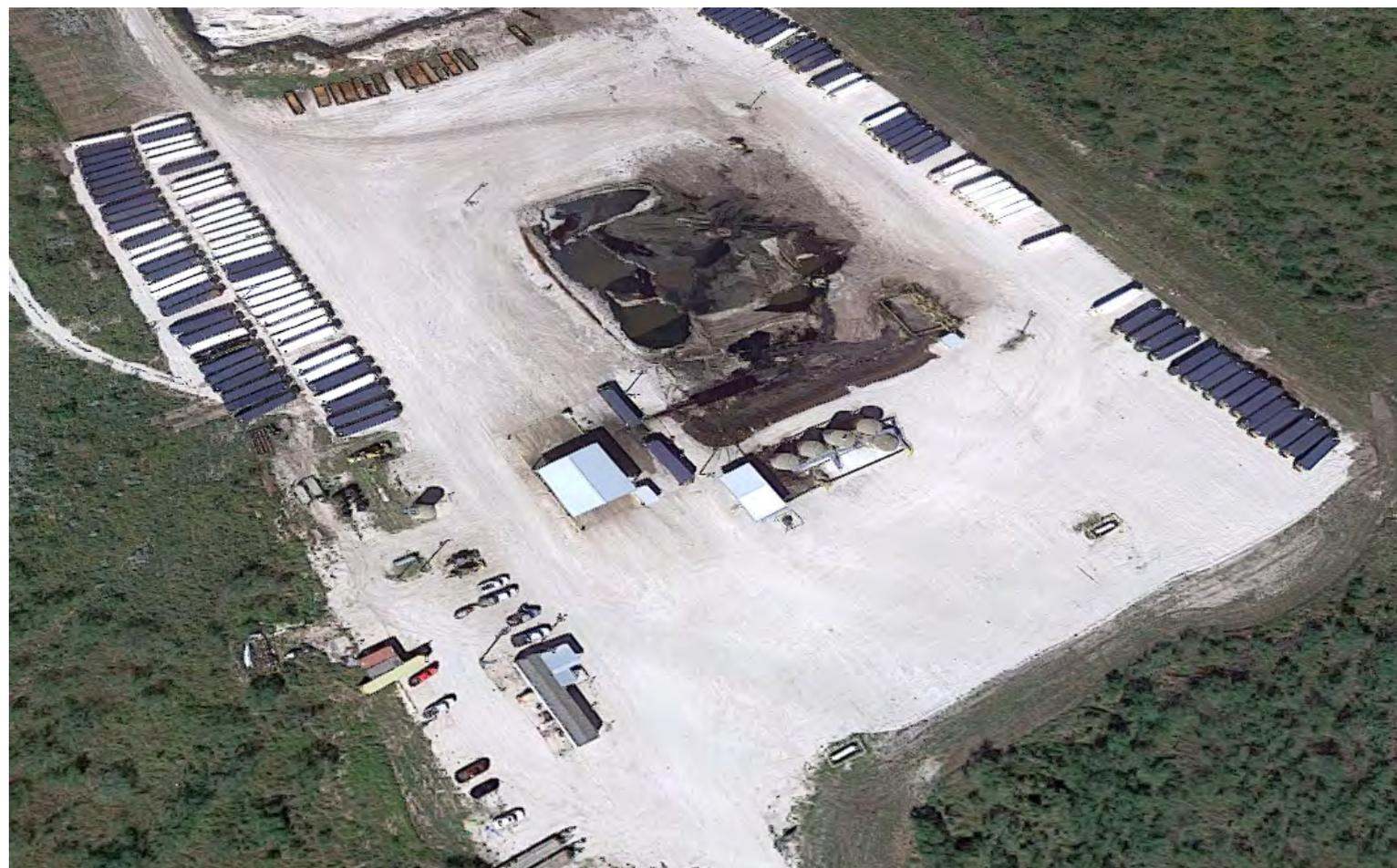
Built on a former caliche mine, the Blackhorn Environmental Services oil and gas waste disposal facility includes pits to separate solid and liquid material and other pits where waste is dried before being dumped in disposal cells. Credit: Google.
