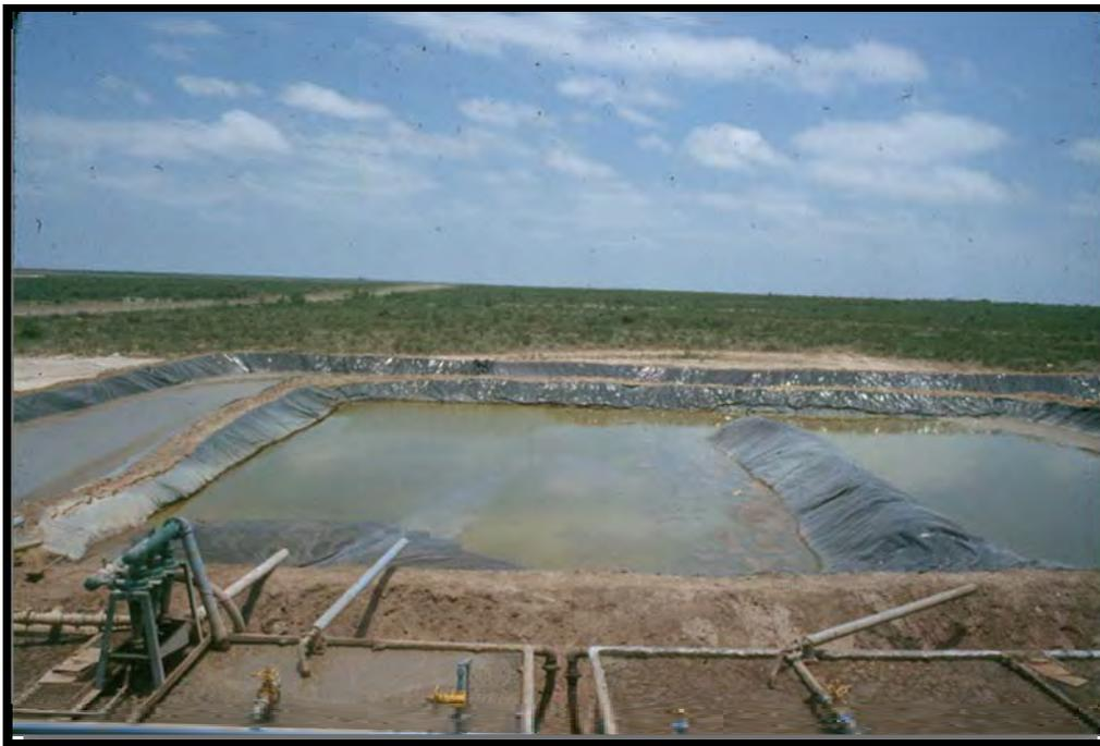
**Photo 2. Oil well reserve pit containing drilling fluids.**
