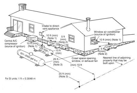
**Note 1:** Regardless of its size, any ASME container filled on site must be located so that the filling connection and fixed maximum liquid level gauge are at least 10 ft. from any external source of ignition (e.g., open flame, window A/C, compressor), intake to direct-vented gas appliance, or intake to a mechanical ventilation system.
