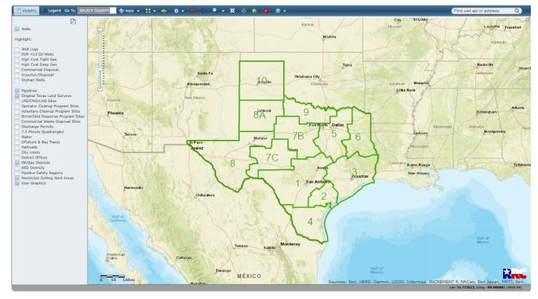
GIS uses polygons, lines and points to depict features. These are graphical representations of real-world items like oil wells, gas pipelines, and alert areas. In the RRC Public GIS Viewer, oil and gas wells are represented as points, pipelines are represented as lines, while district boundaries and alert areas are represented as polygons.
