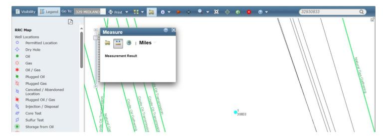
Click on the well to open activate the Measure tool. Move your cursor to the well labeled 31810 directly north. Double-click on the well labeled 31810. This closes the measuring between the points and will show a small green flag at the starting point and the ending point.
