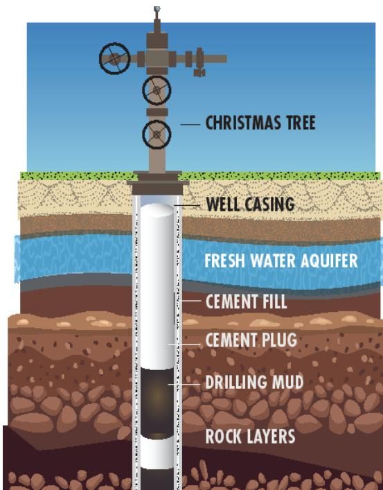
When a well ceases production and no longer produces oil or gas, most operators fulfill their obligations and responsibly follow the required regulatory procedures to plug their wells with cement to prevent the well from leaking and polluting land or groundwater. However, if the operator is noncompliant or goes out of business, the well becomes orphaned.
