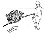
WRONG WAY-When dry chemical is shot into the center of fire, the fire continues to burn. RIGHT WAY-Immediate extinguishment is achieved when dry chemical stream is directed at source of fuel through to the base of the fire.
