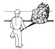
**Figure 1b** Right Way and Wrong Way to Handle Small LP-Gas Fires
