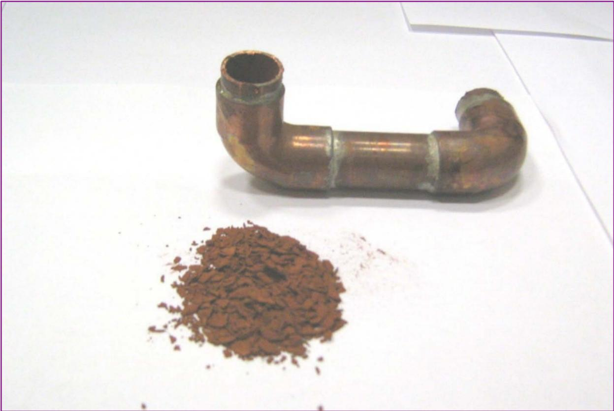
*Loose scale inside the elbow of the tankless water heater using unsoftened water*
